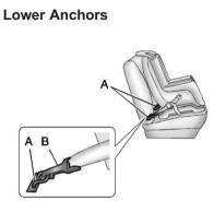
Lower anchors (A) are metal bars built into the vehicle. There are two lower anchors for each LATCH seating position that will accommodate a child restraint with lower attachments (B).
